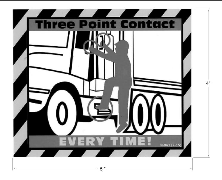
THERE SHALL BE A PERMANENT DECAL AFFIXED BY EACH ENTRY POINT. THE SAME PERMANENT DECAL SHALL BE AFFIXED BY EACH LADDER, PLATFORM OR STEP DESIGNED TO BE CLIMBED OR STEPPED ON. MEASUREMENTS OF DECAL ARE REFERENCED ABOVE.
